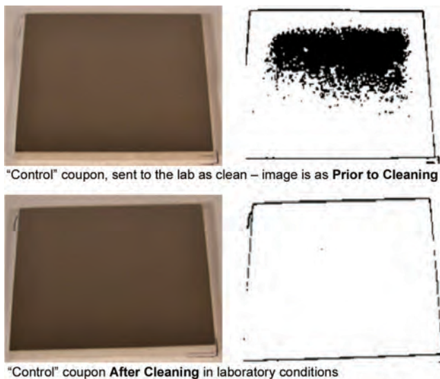
Figure 10. Method Sensitivity – confirming cleanliness on control coupons.
