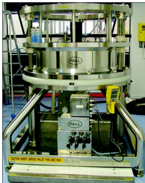
Figure 1. Chromatography columns of 100 cm diameter are routinely used for biopharmaceutical production. Technology transfer and process scale-up may present a number of additional technical challenges (Used with permission from Process Development (Scale-Up) Group, Protherics UK Ltd.)
