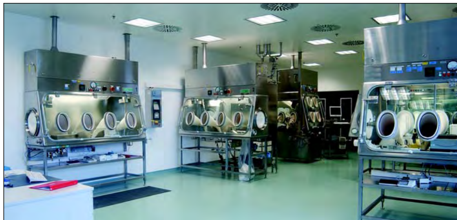
Isolator suite for highly potent compounds/small scale operations.
