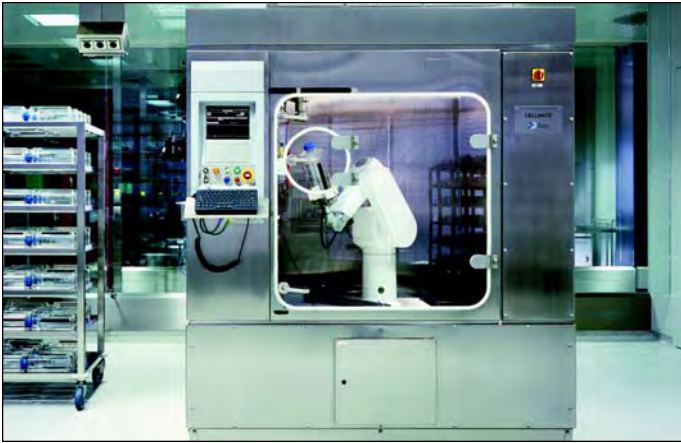
Fully automated roller culture for virus production using robots.
