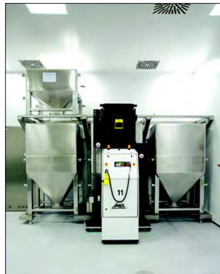
AGV transport system for bins in manufacturing cell.
